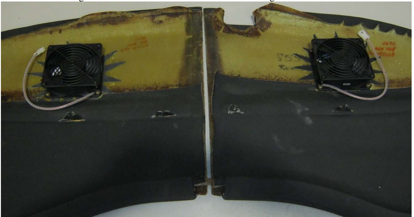
Figure 2. Bottom View of Glare Shield Fan Installation
