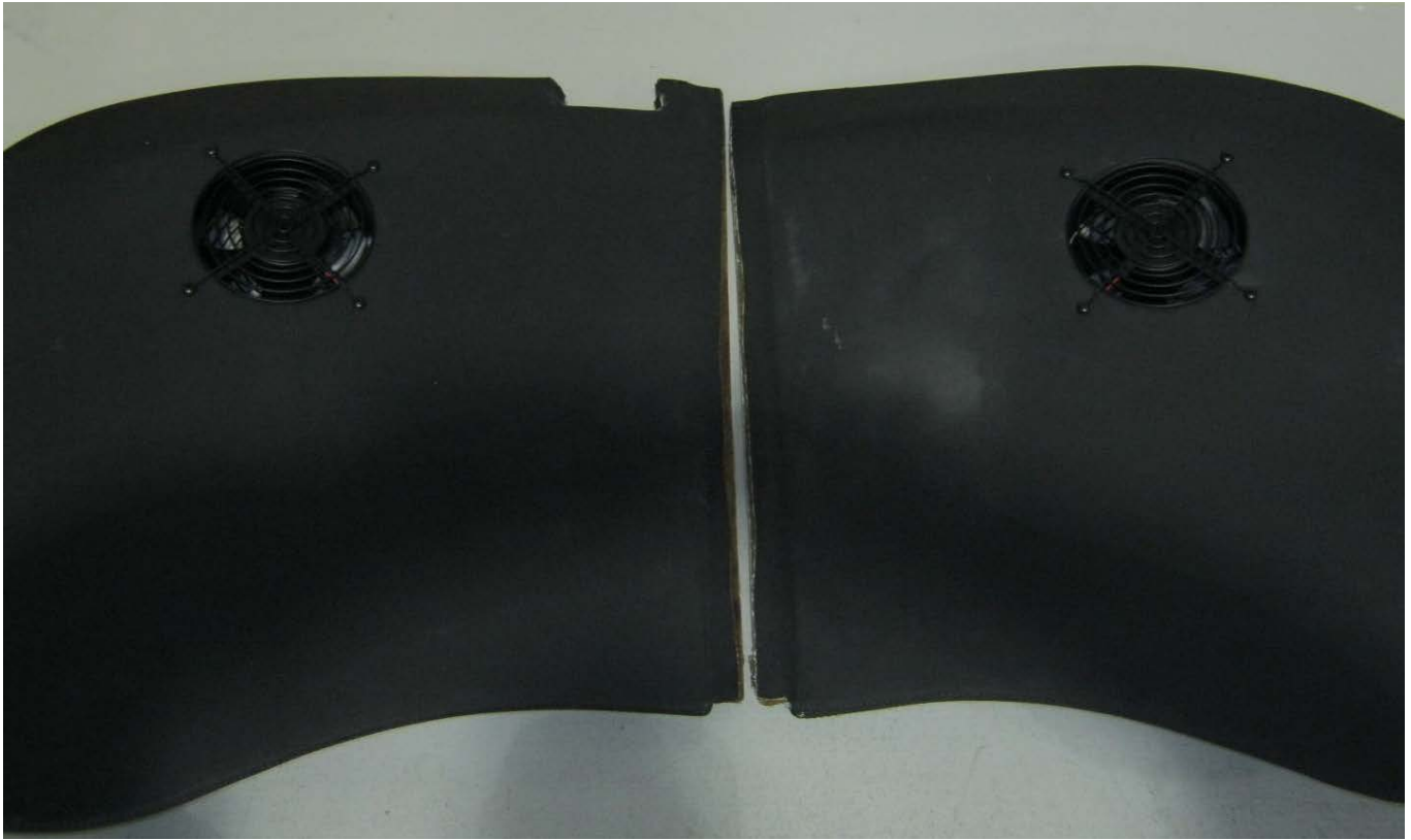
Figure 1. Glare Shield Fans Installed in Left and Right Glare Shields
