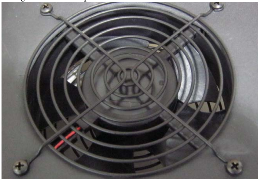
Figure 4. Close Up Top View of Glare Shield Fan Installation
